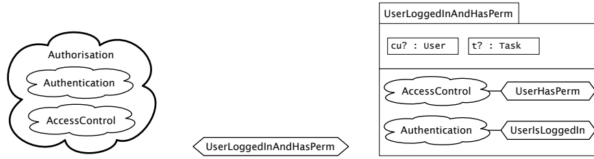
Fig. 25. Package Authorisation extends Authentication and AccessControl (left). Authorisation’s behavioural diagram (centre). Constraint diagram defining behavioural constraint UserIsLoggedInAndHasPerm.
