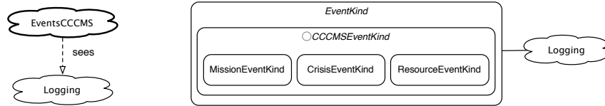
Fig. 42. Package EventsCCCMS extends Logging (left). EventsCCCMS's SD specialise blob EventKind defined in Logging (right).
